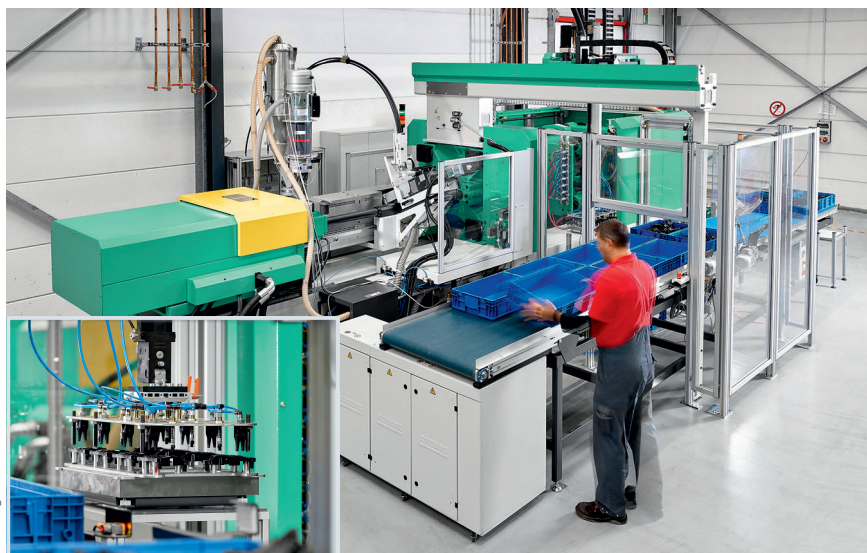
Fig. 2. The FDC system manufactures parts such as cable drive housings made of PP-GF30. After the removal the robotic system sets them down on a scale to check the correct glass fiber content
